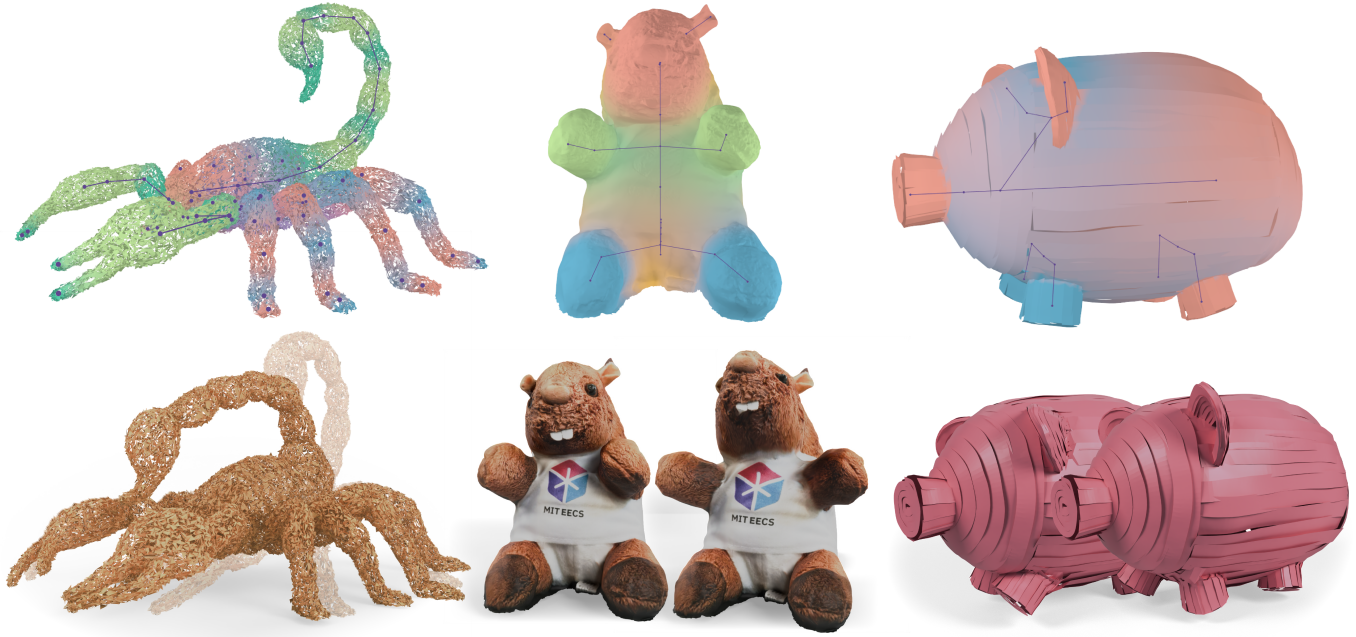
Fig. 1. Bounded biharmonic weights produced by our method can be used to extrapolate color (top row) or deformations (bottom row) from control handles. Our method succeeds on meshes that are typically difficult to handle with standard tools. As an extreme example, the SCORPION (RANDOMIZED) triangle soup is missing 30% of its faces and has had the remaining ones randomly perturbed. We can robustly compute weights for meshes created using off-the-shelf 3D scanning software even if they are non-watertight and contain thin and self-intersecting triangles as does the BEAVER mesh. Similarly, our method can be used to deform virtual reality ribbon drawings [Rosales et al. 2019], such as the PIGGYBANK mesh.
