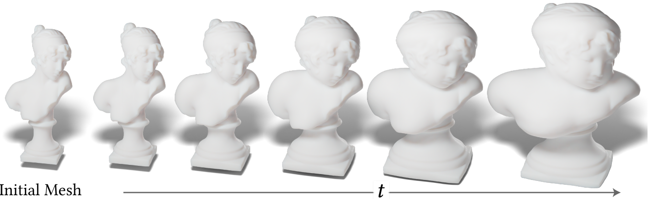
Fig. 3. Mesh inflation via inverse mean curvature flow. The SAPHRO mesh is inflated by treating it as the solution to the mean curvature flow at some time t and optimizing for the initial condition that led to that solution. Larger t results in more inflation.
